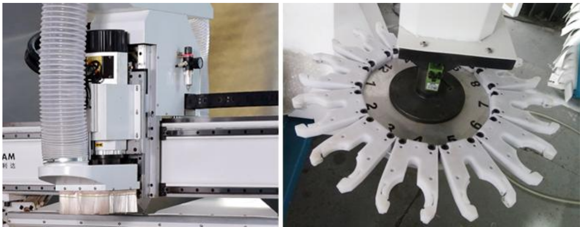
9.0kw ATC spindle with circle tool magazine that could change 12 tools automatically.
